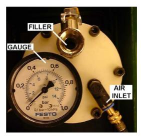
The Ardmel Mini Hydrostatic Head Tester has been designed as a simple to use, portable and cost effective water penetration test machine.
